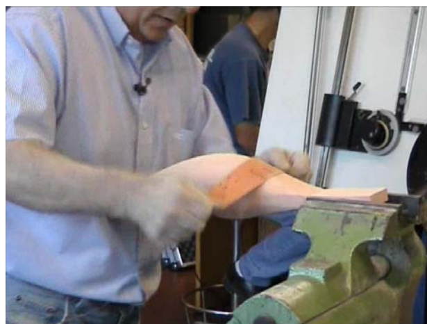
Figure 22. – Modeler performing finishing actions using sand paper (courtesy of Alessi).
