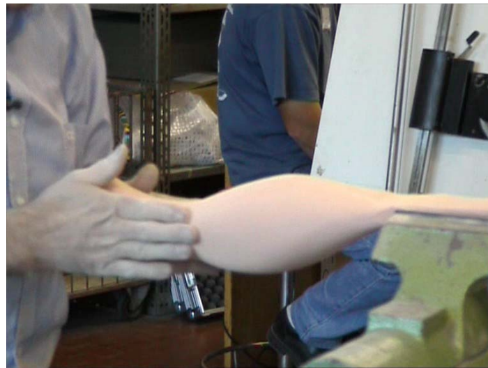
Figure 21. – Modeler performing quality checking actions using hands (courtesy of Alessi).
